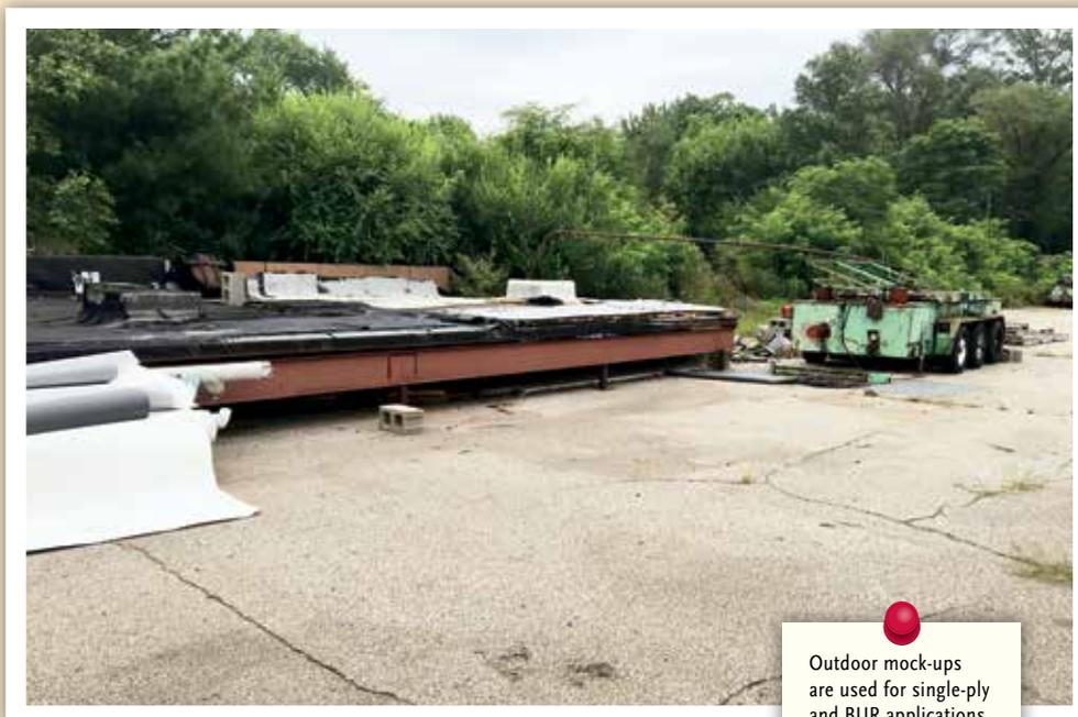
Outdoor mock-ups are used for single-ply and BUR applications.
