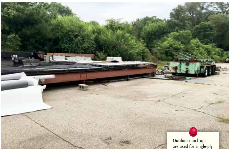
Outdoor mock-ups are used for single-ply and BUR applications.
