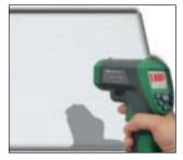
The 'cool roof' curriculum explains what make cool roofs 'cool.' Above, an infrared gun measures the heat reflected from two types of roofing materials in 89° F ambient air. The EPDM single-ply at left is 173°F. A cool coating over BUR at right yields a reading of 108°F.
