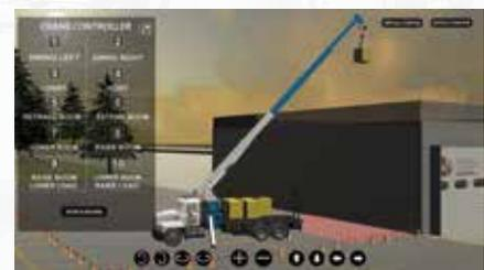
The Signal Person/Crane Interactive Tool is a computer-based program that allows instructors and students to signal and operate a simulated crane as it delivers material onto a rooftop.
