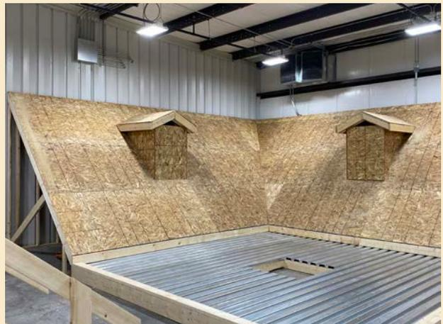
Slate, tile and low-slope mock-up
