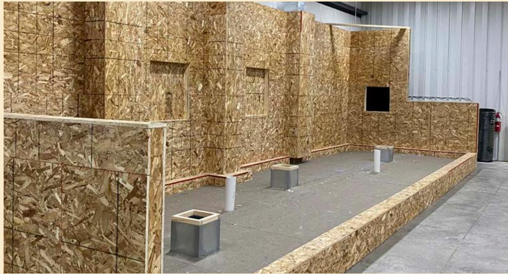
Waterproofing and air barrier mock-up
